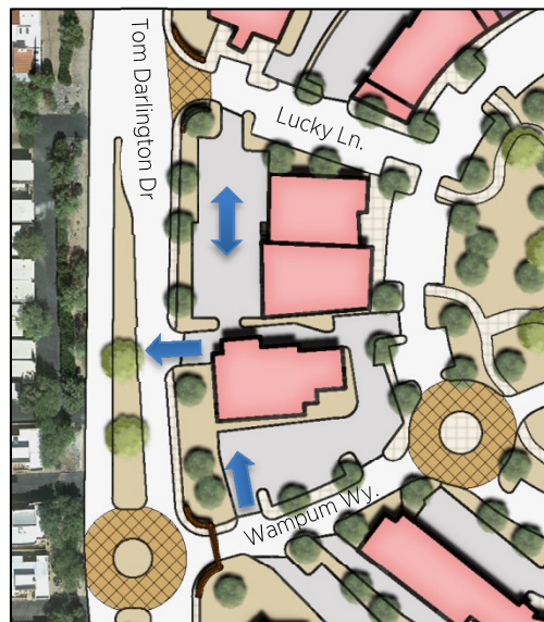
Conceptual Rendering: Creating cross-access connections and relocating entry drives to side streets reduces the number of entry drives along Tom Darlington Drive and helps encourage visitors to utilize desired primary access points when entering the Village Center.
